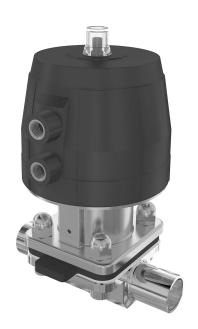
Series 25 pneumatically operated diaphragm valve has a flow-optimized stainless steel body, a diaphragm, and actuator. The stainless steel body is available with various surface finish.
