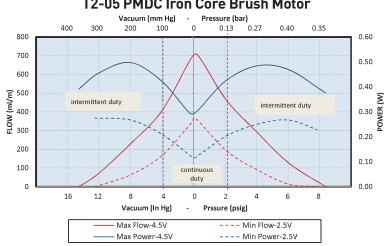
The above graphs represent examples of performance for the pumps series handling air at 800 feet (244M) above sea level at 75° F (24° C). Performance will vary depending on barometric pressure and media temperature. Curves are representative of standard pump configurations. Pump configurations could be customized for higher or lower flows, depending on specific customer requirements.
